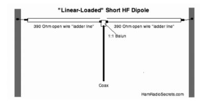
This page describes a way to build a linearly-loaded dipole antenna with a feed point impedance of approximately  $35~\Omega$ . This allows you to feed it with coax instead of the ladder line that I use. The author uses  $390~\Omega$  ladder line for the elements. He says it's commonly available, but I don't think I've ever seen  $390~\Omega$  ladder line. You could probably use  $450~\Omega$  ladder line by adjusting the element lengths a little.
